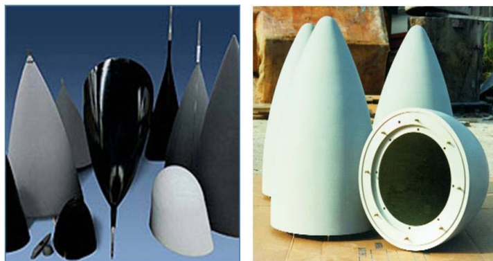
Left: a selection of aerodynamic radomes (Northrop Grumman). Right: radomes similar to those that might be used to protect RV seekers on reentry. (American Technology & Research Industries)
