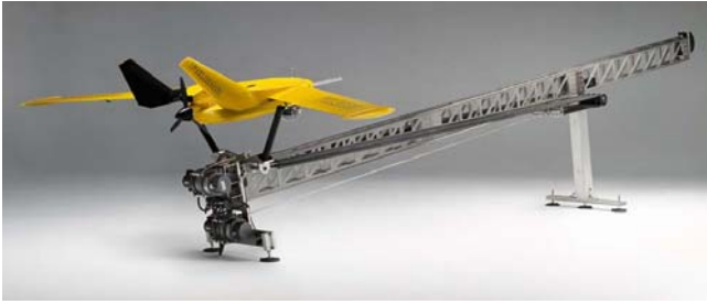
A medium-range endurance UAV. Despite its small size, this elastic catapult-launched UAV is capable of carrying a 1 kg payload (IR and digital cameras) to a range of 400 km. (Aerovision Vehiculos Aereos, SL)
