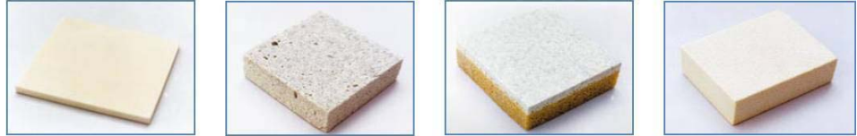
Four radar absorbing material foams, clockwise from upper left: low-dielectric foam (epoxy); lightweight lossy foam (urethane); sprayable lightweight foam (urethane); and thermoplastic foam (polytherimide). (MTCR Equipment, Software and Technology Annex Handbook, Third Edition (May 2005))
