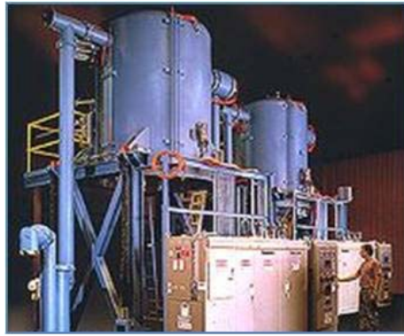
Left: A large scale custom CVD furnace which inductively heats graphite to temperatures in the 2800 °C range. (CVI)
