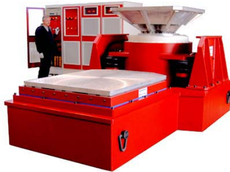
An example of a thruster with slip table. (Kingdom Pty Ltd)
