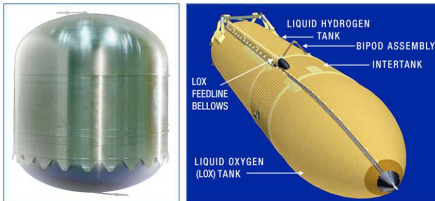
Left: A typical liquid propellant tank developed for a range of space applications. (EADS) Right: A diagram of the external tank used by a space vehicle launch engine, showing the separated oxidizer and fuel tanks. (NASA)
