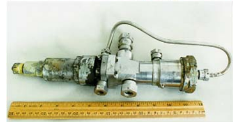
Top Right: A multi-shaft turbopump assembly. (Aerojet) Top (far) right: A single-shaft turbopump. (Aerojet) Bottom: A servo valve from a Scud missile. (MTCR Equipment, Software, and Technology Annex Handbook, Third Edition)
