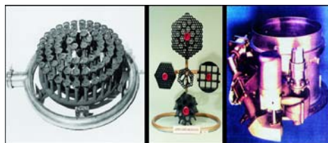
Left: A fuel manifold and centrifugal fuel injector assembly for a ramjet engine. (Kaiser Marquardt) Center: Various aerodynamic grids used to straighten the flow of air into a ramjet engine. (Kaiser Marquardt) Right: A fuel management system for a ramjet engine. (Kaiser Marquardt)
