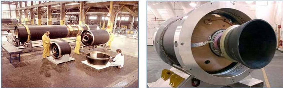
of mission platforms, including the first, second and third stage rocket stages of space launch vehicles. (ATK) Right: A rocket motor – installed in a rocket case – which functions as the motor in the third-stage of a launch vehicle. (ATK)
