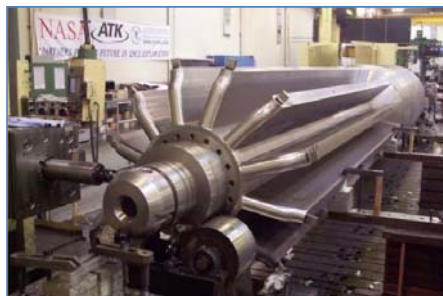
Figure 1: A propellant casting mandrel. (ATK)
