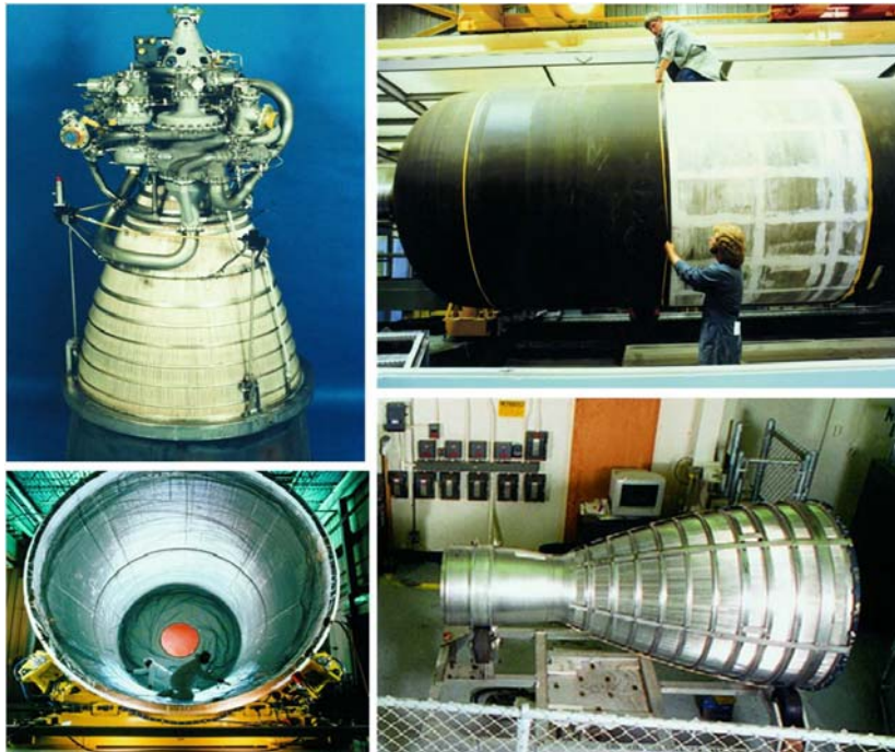
Top left: An engine with a large, regeneratively cooled nozzle. (MTCR Equipment, Software and Technology Handbook, Third edition (May 2005)) Bottom left: Installation of insulation inside a filament wound rocket motor case. (Thiokol Corp.) Top right: A rocket motor case under inspection after application of the thermal insulation. (Fiat Avio) Bottom right: Side view of a regeneratively cooled nozzle. (Boeing)
