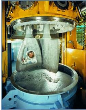
Figure 5: Solid propellant being mixed in a 600-gallon vertical planetary mixer. (Thiokol Corp.)
