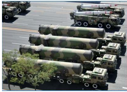
Eight axle and four axle TELs carrying intercontinental ballistic missiles (ICBMs; foreground) and intermediate range ballistic missiles (IRBMs). (Via Chinese Internet)
