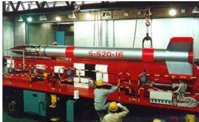
A large Category II sounding rocket, capable of delivering a 250 kg payload to a range of 400 km. The rocket’s solid propellant motor, with steel casing, is surrounded by four honeycomb tail fins with titanium alloy leading edges. (JAXA)
