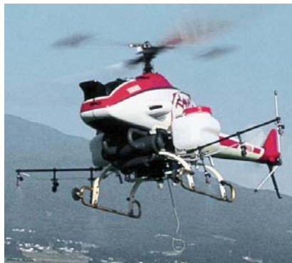
A rotary-wing UAV designed with chemical tanks and spray bars for agricultural purposes. (Yamaha)
