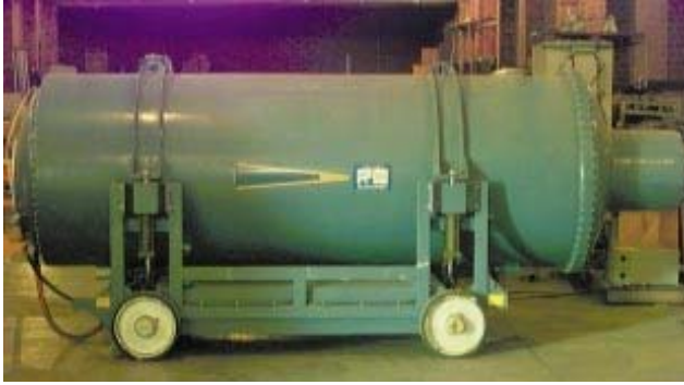
A 2.3MeV flash X-ray unit used for inspecting solid rocket motors. (MTCR Equipment, Software and Technology Annex Handbook, Third Edition (May 2005))
