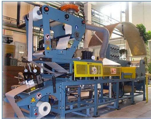
A prepreg machine constructed by the Composite Materials Group for the production of prepreg materials using fibers and resins. (Katholieke Universiteit Leuven)
