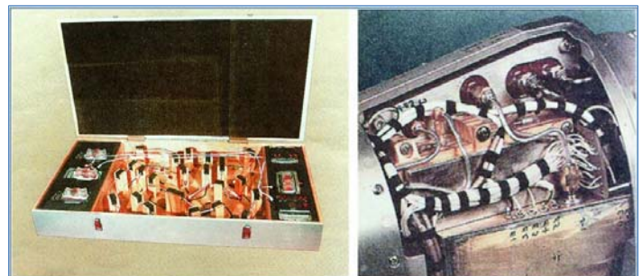
Figure 6: Left: An RV radar antenna set packaged for shipment. Right: A portion of RV radar electronics. (MTCR Equipment, Software and Technology Handbook, Third edition (May 2005))
