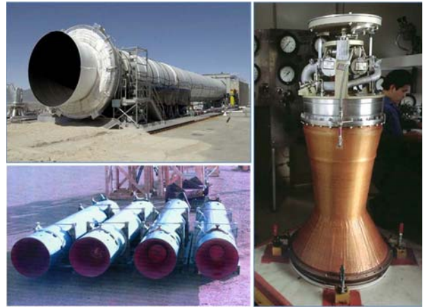
Figure 7: Top left: A re-usable solid rocket motor for space vehicle use. (ATK) Bottom left: Solid propellant rocket motors with total impulse close to the lower limit of Item 2 control. (MTCR Equipment, Software and Technology Handbook, Third edition (May 2005)) Right: A pressure-fed liquid rocket engine. (Aerojet)
