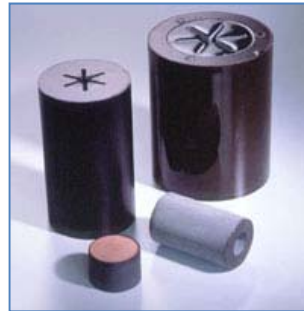
Figure 7: Composite propellants manufactured for use in rocket motors. (Daicel Chemical Industries, Ltd)
